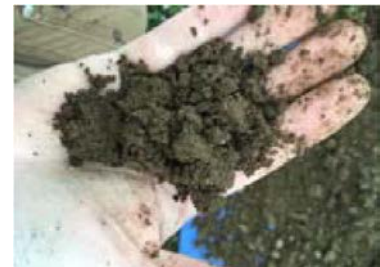
Figure 16. Soils at the Berlin Elementary School were generally a mix of silt and sandy.
