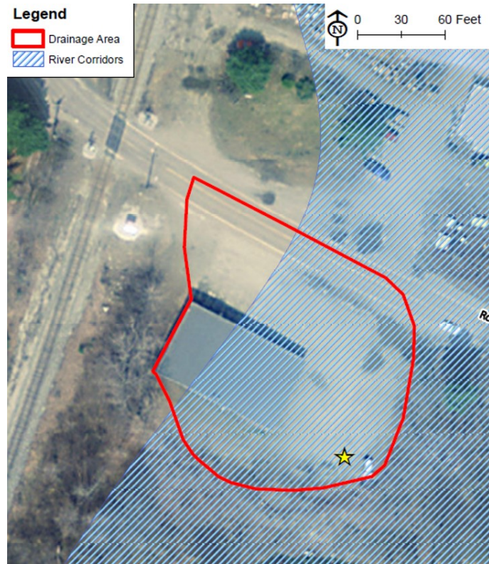
Figure 20. The proposed infiltration trench is located in the southeast corner (see starred location) of the Berlin Fire Department 1's drainage area, which is shown in red.
