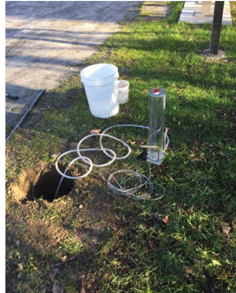
Figure 14. An example of the Constant-Head Borehole Permeameter Test in progress using a Johnson Meter.
