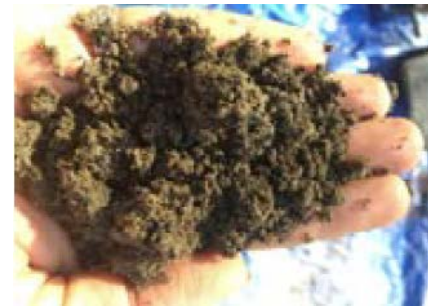
Figure 21. Soils at the Berlin Fire Department 1 site were generally a mix of sand and gravel.
